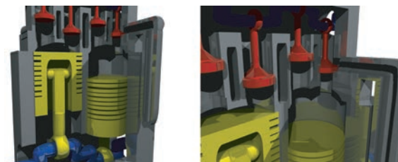
Fig. 17. Constructive modeling examples built using our new operators. In this model, clean union and clean difference operators have been used in conjunction with gradient-based blending operators. Both sharp edges and subsequent gradient-controlled blends have thus been efficiently performed.
